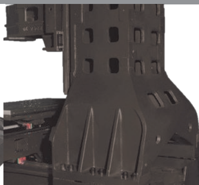
Reinforced ribbed cast iron
