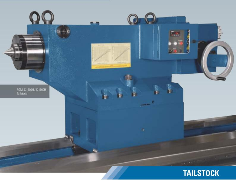
The manually driven quill has a built-in live center with high precision bearings. It has a monitoring system by load sensors of the thrust force. Its displacement is driven by gearmotor and pinion /rack system.
