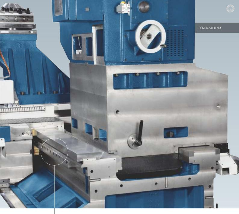
Rack (Güdel) of the longitudinal saddle displacement system.
