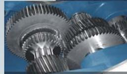
Gears from the headstock transmission system with hardened and ground teeth, designed to withstand the high efforts of the most severe working conditions.
