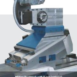
Milling Headstock with Y axis (optional) Spindle taper ISO-50, 16 hp / 12 kW, 2,500 rpm (max.)
