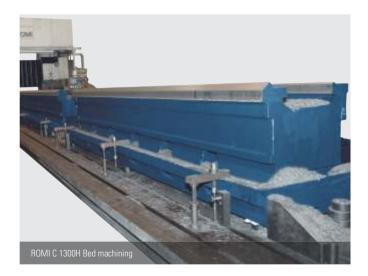
Robust monoblock bed made of gray cast iron. Offers great rigidity, absorbing high machining efforts and vibration, assuring stability and accuracy at full power operation. The bed is a base for components supporting and it is fixed on the foundation by levelling and alignment elements.
