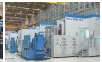
Flexible Manufacturing System
