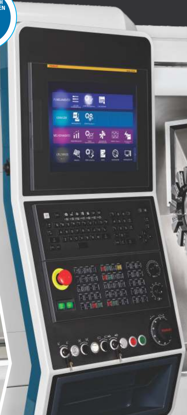
Fanuc 0i-TF i -HMI CNC (for T, M and Y versions) with 15" Touchscreen LED color monitor
