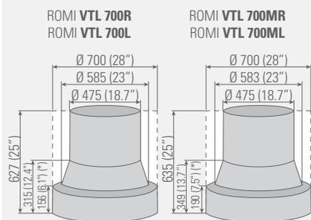
(\* Interference area when working length exceeds 156 mm (6.1")
