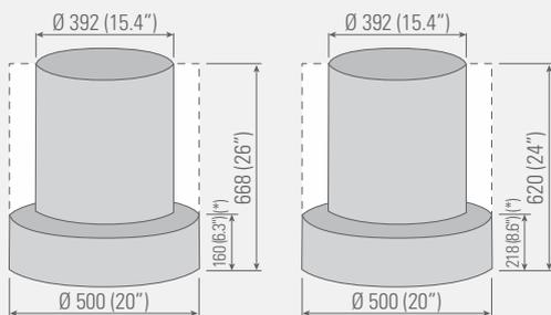
(\*) Interference area when working length exceeds 160 mm (6.3")
