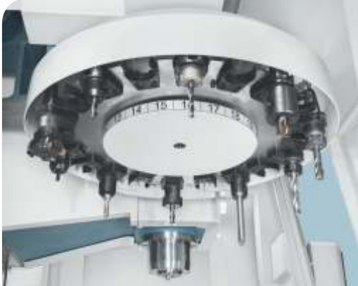
Automatic Tool Changer with 20 tools capacity (ROMI D 600)
